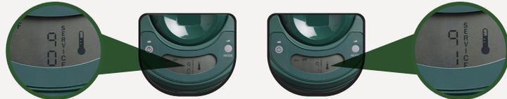
1.4 - Press both MODE and POWER buttons for 10 seconds - the screen will display "90" and "91" alternatively.
