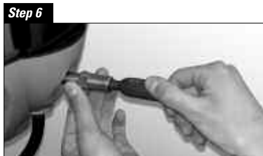
Step 6 To start cleaning process, while holding Quick Clear adapter in place, unscrew the Quick Clear cartridge 1/4 Turn Only .
