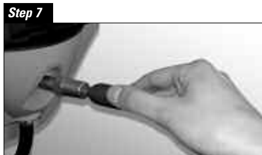
Step 7 Unscrew the Quick Clear cartridge first, then unscrew Quick Clear adapter and discard the spent Quick Clear cartridge. Remember to keep the Quick Clear adapter for future use.
