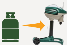
2.3 - Connect a full 20 lb. propane tank.
