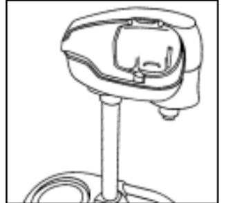
Completed assembly should have the front of power head in the same direction as base U-shaped legs.
